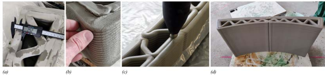
Figure 114 – Material tests and prototyping. (a) Path and infill tests. (b) Defining material and processing parameters for consistency. (c,d) Learnings had been reintroduced for the final design, most relevant being the seam details for the deck blocks.
