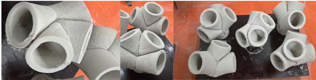
Figure 77 – Materially bonded, compound 3DCP objects. Photographs showing various types of nodes that vary in valence and angles between incident edges.
