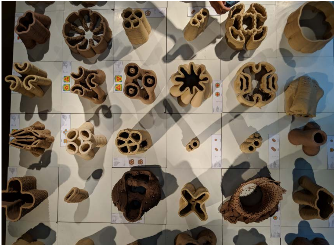
Figure 71 – Bifurcating tubular topology shape design results. Results produced by first-time user, architectural students during a 5-day design-to-production workshop (“digitalFutures,” 2018).
