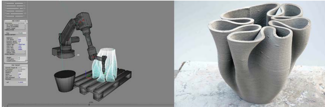
Figure 67 – Post-processing of print paths by 3D concrete Printing (3DCP) manufacturer (“Incremental3d,” 2017). (Left) Processing of an outcome produced by proposed IDE by the manufacturer. (Right) Prototype demonstrating the application of the proposed method.
