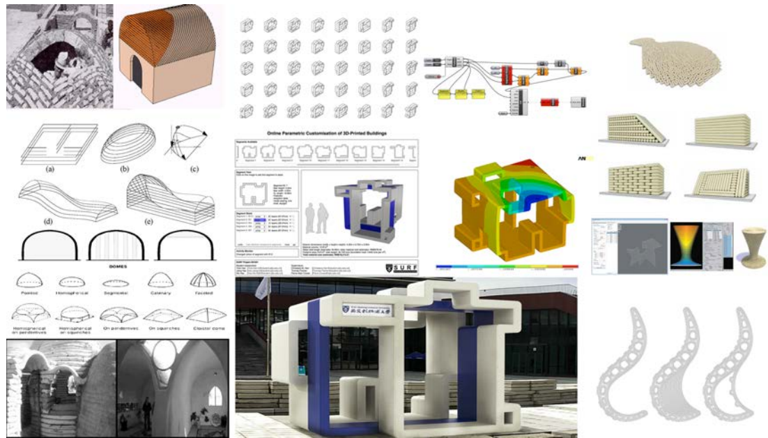
Figure 13 – Prior design explorers for 3DCP. (Left column) Designer handbook and other aspects of funicular shell design considered relevant by Contour Crafting® 3D printing company (Khoshnevis et al., 2006a). (Middle Column) Parametric design exploration of feasible designs, online customization interface, structural analysis and realised result by tutors and students of Xi'an Jiaotong-Liverpool University (Chien et al., 2016). (Right column ) Design tools developed by Foster and Partners and Loughborough University to slice existing geometries and explore toolpaths of the 3d Printer and resultant geometries (De Kestelier and Buswell, 2009).
