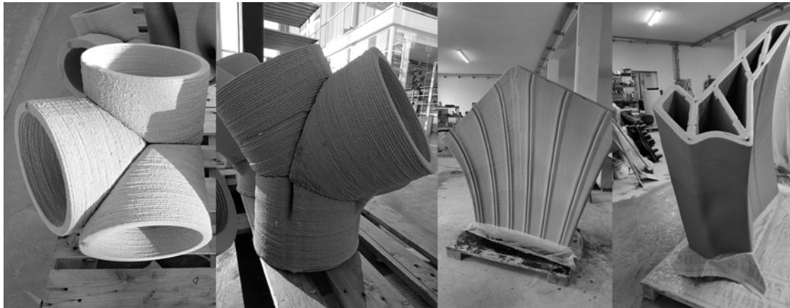
Figure 9 – Photographs of a force-aligned, inclined-plane 3DCP of components of funicular structures
