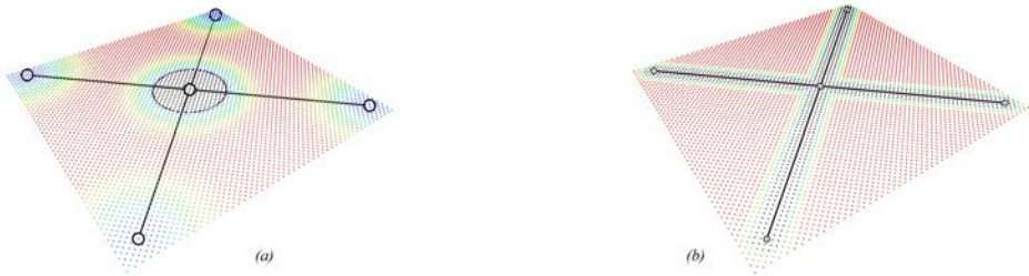
Figure 39 –Signed distance fields (SDF). (a) SDF in relation to the nodes of a skeletal graph. (b) SDF in relation to the edges of a skeletal graph.
