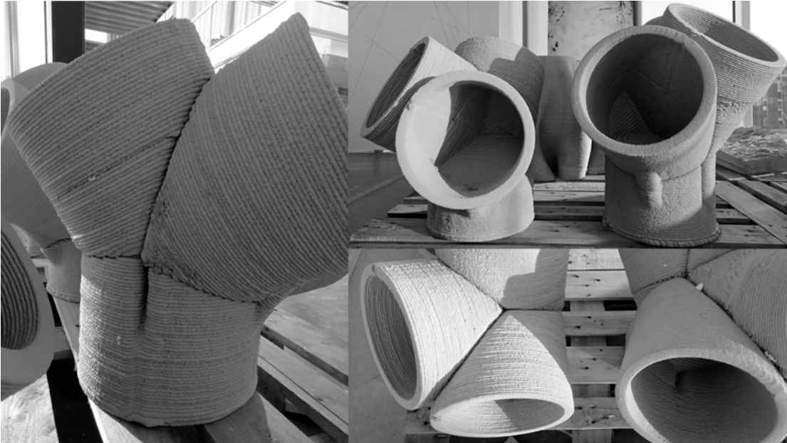
Figure 78 – Force-aligned, inclined-plane 3DCP of a node in a funicular skeleton.
